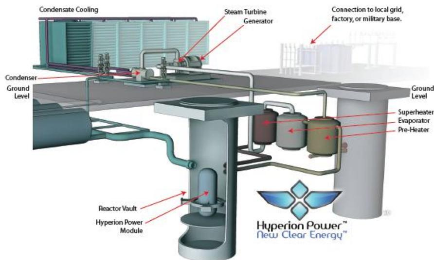
*Hyperion Power Module-based 25MWe Electric Power Plant*
